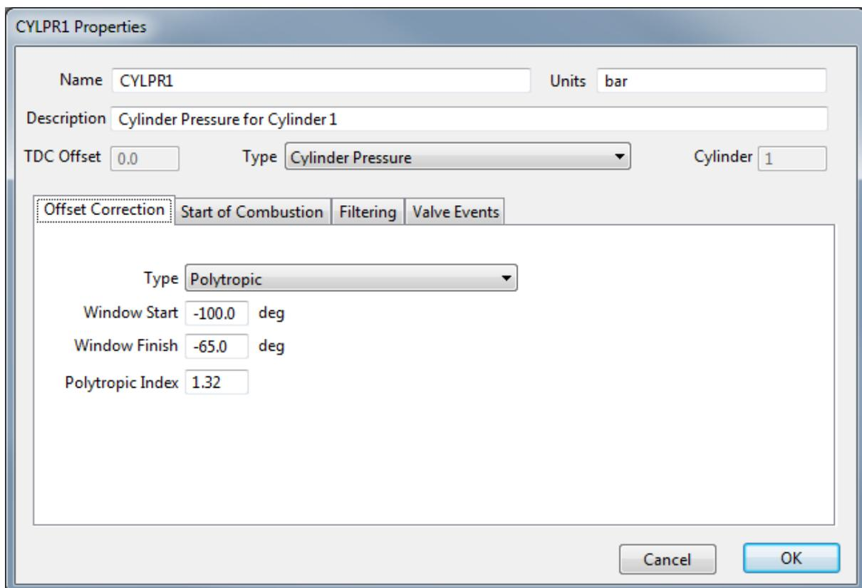
The image shows a software dialog box titled "CYLPR1 Properties". It contains several input fields and a tabbed interface. The "Offset Correction" tab is selected, showing a "Type" dropdown set to "Polytropic", a "Window Start" of -100.0 deg, a "Window Finish" of -65.0 deg, and a "Polytropic Index" of 1.32. Other tabs include "Start of Combustion", "Filtering", and "Valve Events".
